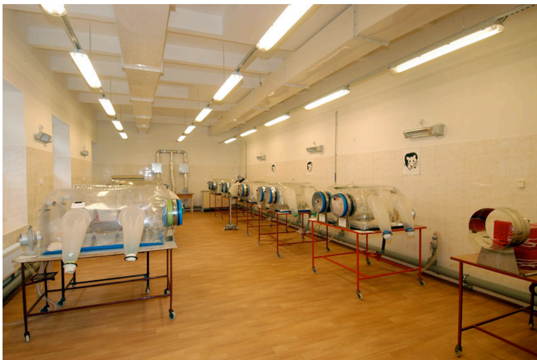
Figure 1: Germfree or Lactobacillus plantarum -monocolonized mice were reared in Trexler-type isolators in the Laboratory of Gnotobiology, Institute of Microbiology, Academy of Sciences of the Czech Republic in Novy Hradek.
